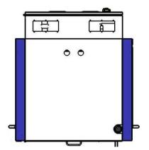
main supply: 1x230 Vac 50-60 Hz CEE17 16A socket power consumption: max 12 A compressed air 6Kg/cm² connection LAN & USB socket collector for external fume extraction ESD bracelet socket Sinergo software license
