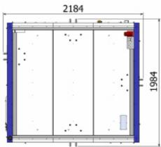
main supply: 3x400 Vac 50-60Hz power consumption: max. 10 Kva 3 poles + GND socket 32A CEE IEC309 compressed air 6Kg/cm2 connection LAN & USB socket Sinergo software license panel PC Windows 7 license
